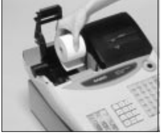
Step 3 Ensuring the paper is being fed from the bottom of the roll, lower the roll into the space behind the printer.
